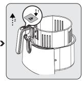
To release the basket from the drawer, place the drawer on a flat surface. Lift the protection cover (5), press the basket release button (6) and lift the basket out of the drawer.
